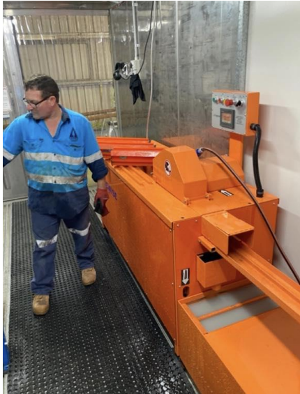
[Figure 6] Automated Core Saw
